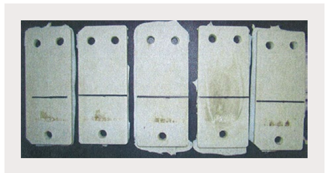
Fig. 8: Material samples after test for the evaluation of the resistance to tracking and erosion
