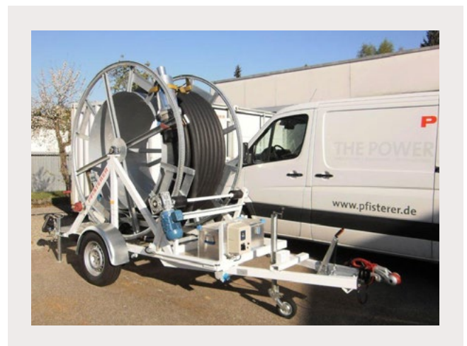
Fig. 17: Cable link on trailer for temporary installation
