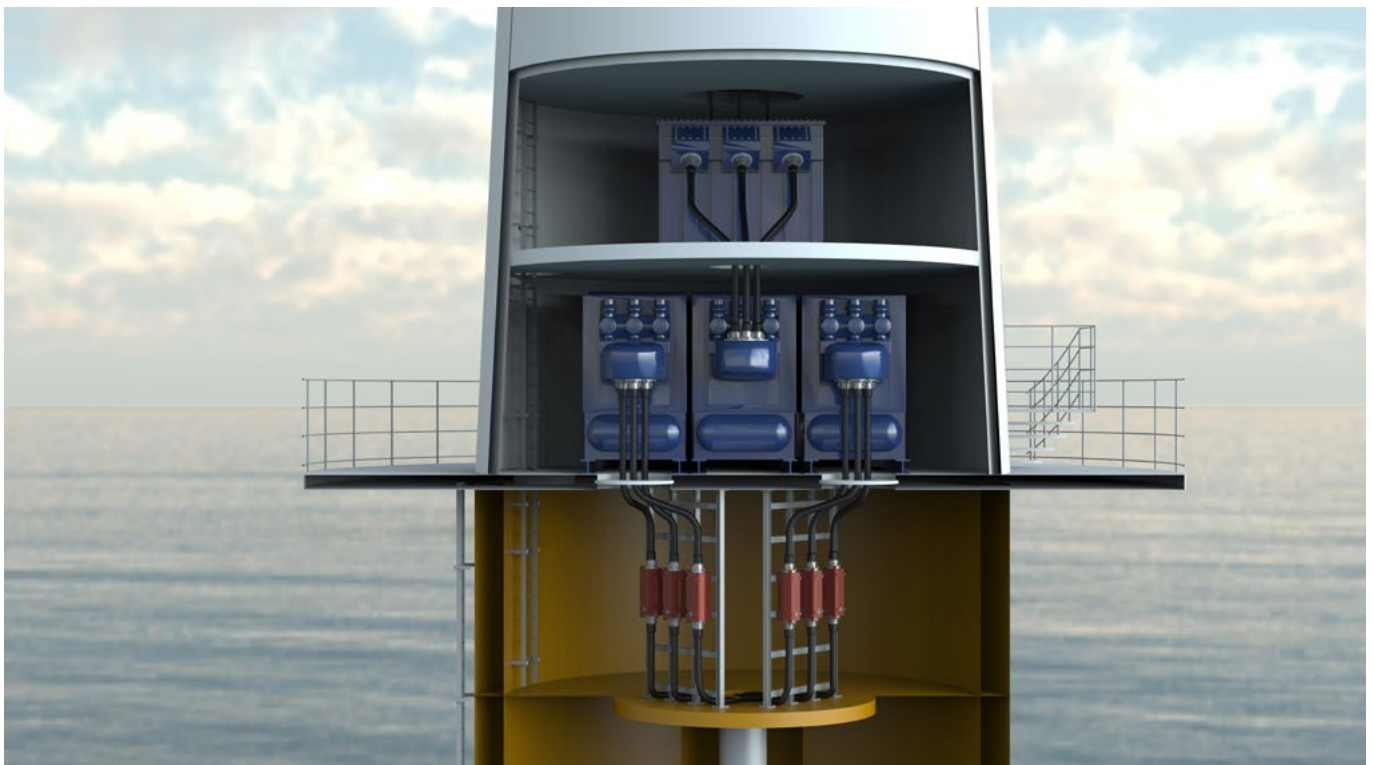
Fig. 9b: Connection between sea and tower cable in an offshore wind power generation application
