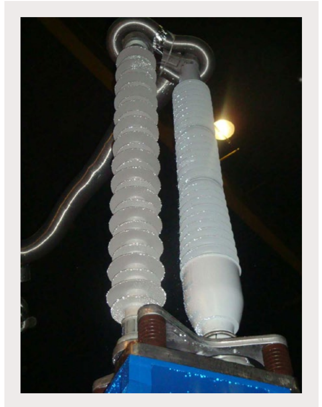
Fig. 7: HV cable termination type EST170-C53L during wet power frequency withstand voltage test
