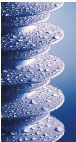
Fig. 10.1: Hydrophobicity of an unpolluted Silicone Rubber surface
