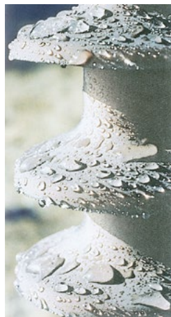
Fig. 10.2: Hydrophobicity after transfer of a polluted Silicone Rubber surface
