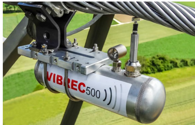
VIBREC500 in operation
